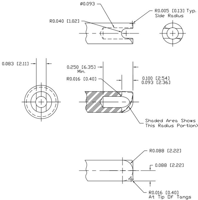
Above is a suggested driver tip design for standard cores, similar features should be used for other core types.
